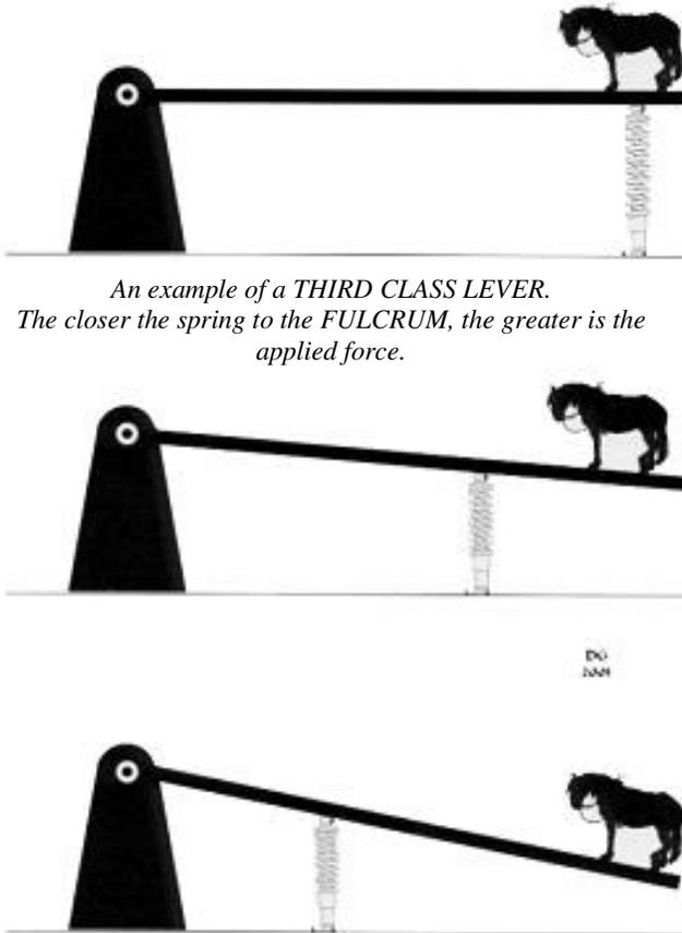
Fig 2: An example of a third class lever.
